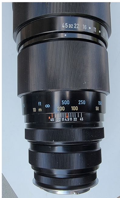
(The apertures range showing f:4.5 to f:45)
